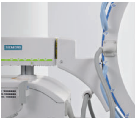
Each moving direction of the C-arm is represented by a color-coded measurement scale
